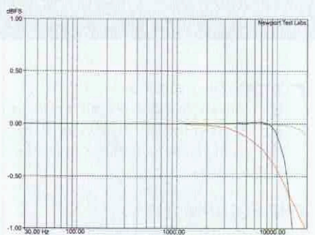
Graph 12: Freq. response showing Super-Slow (red trace), Slow (black trace) and Sharp (green trace) filters.
